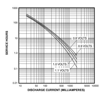
TYPICAL CONTINUOUS PERFORMANCE CHARACTERISTICS WITH CONSTANT CURRENT TO VARIOUS CUTOFF VOLTAGES AT 21 °C (70°F)
